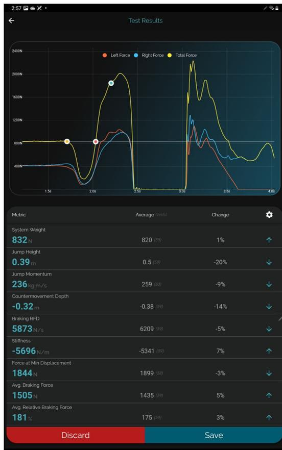
6. Once the test has completed, results will show immediately. To save the test, tap the blue "save" button in the bottom right, and to delete the test click the red "discard" button in the bottom left. You can scroll down and see all the metrics calculated for the test.
